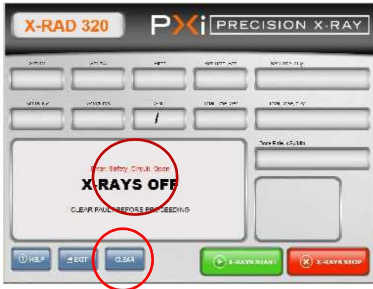
**Note-If an error is present, the User must fix the error and then clear error before producing X-Rays. To clear the error simply select the “CLEAR” button as indicated in the above figure**
