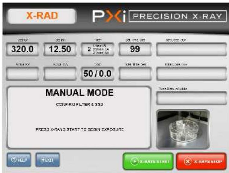
The Specimen Observation System can be viewed in full screen by simply selecting the thumbnail. All crucial X-Ray data is displayed on the lower edge of the screen and includes a “X-RAYS STOP” button in case the user needs to immediately stop X-Rays.
