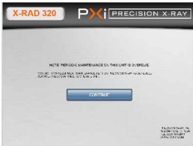
Tapping CONTINUE allows the user to continue to operate the unit, however it will again be displayed every time the unit is powered up until maintenance is performed.
